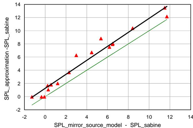
Figure 5: Correlation between the mirror sources model and Eq. (8). Thin line is for an ideal case; the black line is for best fit.
