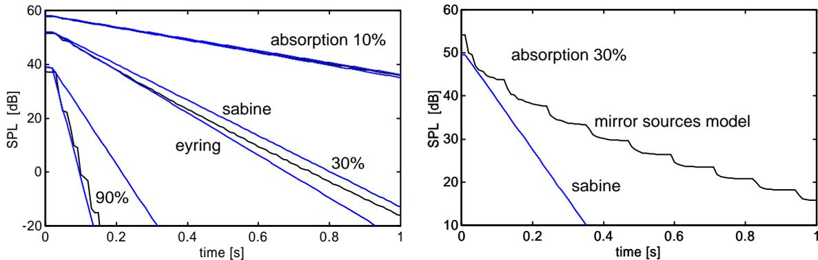
Figure 1: Decay curves for a cubic space of  $10 \times 10 \times 10 \text{ m}^3$  (left) and for a space of  $40 \times 10 \times 2.5 \text{ m}^3$ . Absorption is homogeneously distributed along all surfaces.
