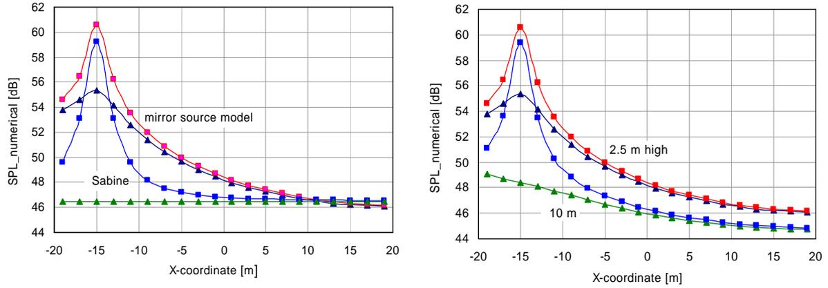
Figure 4: Calculations for a room with  $x$  and  $y$  coordinates ranging from  $-20$  to  $+20$  m. Source position is at  $(-15, -15)$ , the microphone is at  $y = -14$ , while  $x$ -values range from  $-19$  to  $+19$ ; so the shortest distance is  $1$  m and since  $L_w = 70$ , SPL is predicted by common theory as  $59.0$  dB. All surfaces have the same absorption coefficient of  $20\%$ .
