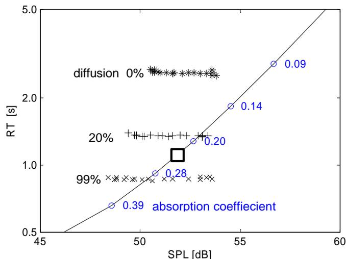
Figure 6: RT and SPL values from a ray-tracing computer model for three different diffusion factors. Room size is  $21 \times 12 \times 5.5 \text{ m}^3$ ;  $\alpha = 0.25$  (small square). There is one source position and 20 microphone positions.
