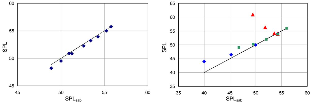
Figure 3: Comparison of the mirror sources model with values from common theory, denoted by  $SPL_{sab}$ . The source power level is taken as 70 dB (re  $10^{-12}$  W). In the left figure all spaces are cubic ( $10 \times 10 \times 10$  m<sup>3</sup>). The basis is the (54.3, 53.9) value where all surfaces have the same absorption coefficient of 20%. Other dots represent a variety of absorption coefficients with 20 / 20 / 99% as an extreme case.
